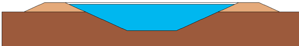
Figure 1. Principle sketch of a pit heat storage cross section.
