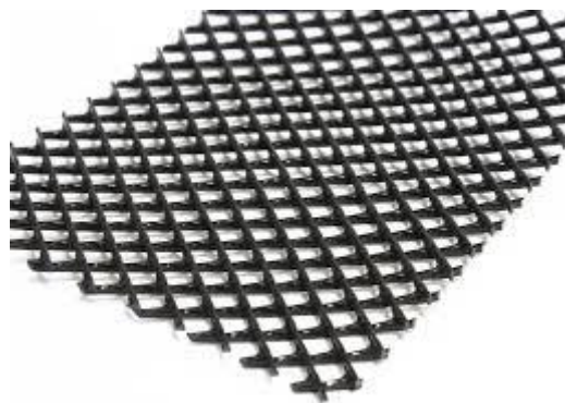
Figure 8. Geonet used to separate the liner and insulation by a small air gap.
